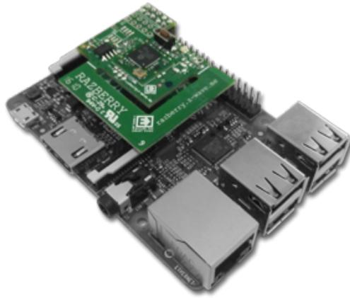
Figure 2.1: RaZberry on top of a Raspberry Pi
