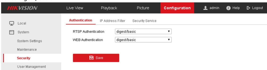
9. You will then need to navigate to Advanced Settings under Network, on the top tabs select Integration Protocol and Enable Hikvision-CGI and Select digest/basic.
